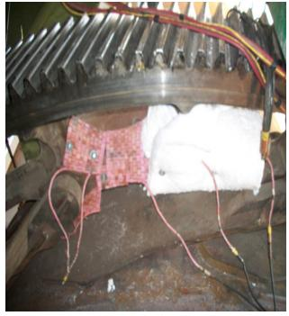
This repair was done in three stages, clean, inspect and secure. Stage 2 was to excavate 50 percent, weld and reinforce. These pictures reveal the bottom plate welded on with a 1 inch fillet weld around perimeter and 50% of the rib excavated and welded in progression.
